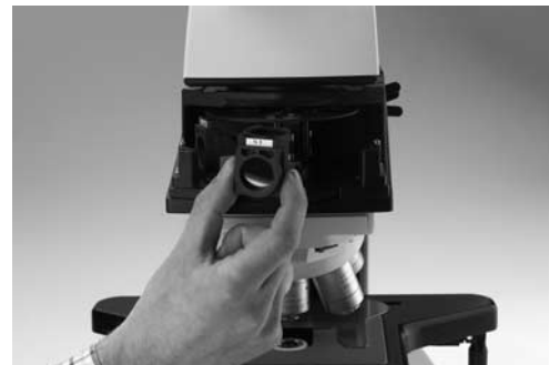
Fig. 25 Mounting the Filter cube
