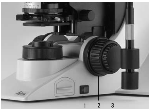
Fig. 51 Focus wheel with flat focus knob 1 Focus stop 2 Coarse focusing 3 Fine focusing
