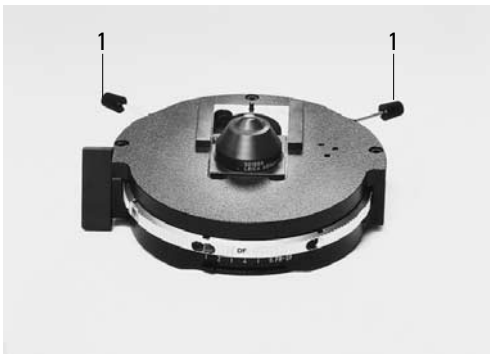
Fig. 38 Light ring centering (i.e.: condenser UCA/P) 1 Centering keys
